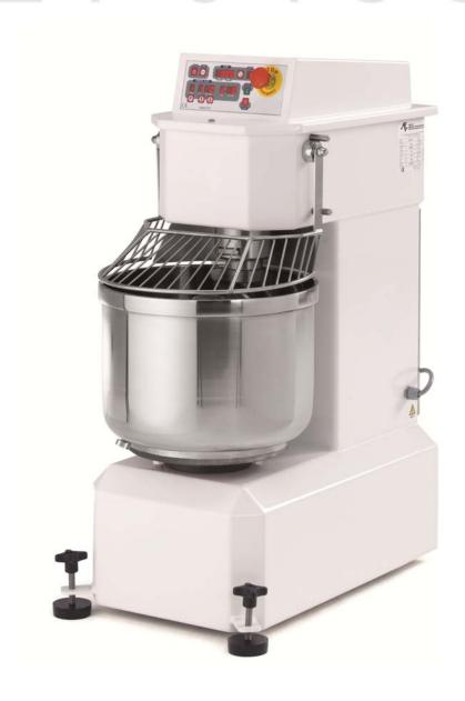
Spiral Mixer, 50 Lb. Dough Capacity, 2 Speeds, Programmable Digital Control, Stationary Stainless Steel Bowl, Safety Guard & Dough Hook, Cast Iron Frame with Enamel Coated Steel Finish, 2 HP, 208-240/60/1P/10A, NEMA 6-15P
